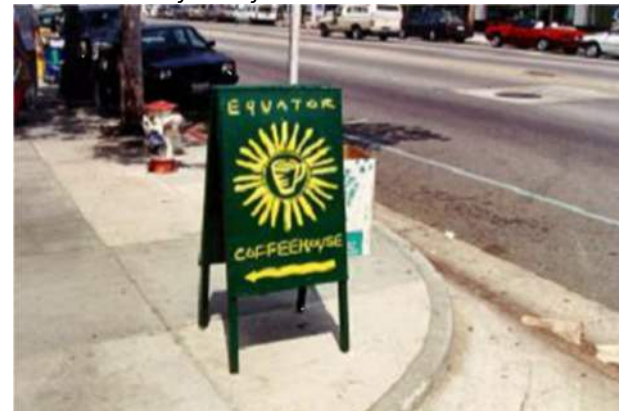
Figure 14.17 This sign is placed too close to the ADA sidewalk, impeding pedestrian cross walk and access.
